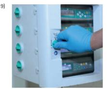
Push the door to close and turn the rotary knob into the horizontal door lock position. Check for acoustic and haptic feedback to ensure that the door is closed.
