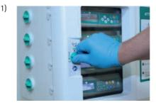
Turn the rotary knob into the door open position and open the door of the SpaceStation MRI.
