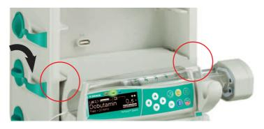
To release, turn the knob clockwise to the vertical position and remove the pump. After release the pump is held in the SpaceStation MRI by the guide rails, but can drop due to bumping or during movement of the SpaceStation MRI.
