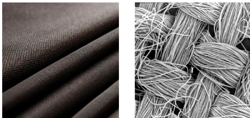
Figure 3. Activated Carbon Cloth Matrix (Zorflex®) in the TOXI-GUARD® system. Left panel, unmagnified picture. Right panel, magnified picture of the active carbon cloth, showing the tight weave of the carbon cloth matrix.
