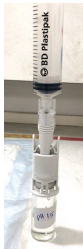
Figure 2. OnGuard ® 2 Syringe Adaptor and BD syringe connected to OnGuard ® 2 Vial Adaptor and vial containing acidic solution
