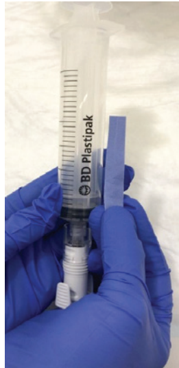
Figure 5. Test results: no color change on litmus blue indicator paper after sampling inner syringe barrels
