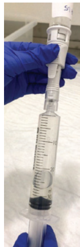
Figure 3. Withdrawal of acidic solution into BD syringe, ensuring contact with all inner walls of the syringe barrel
