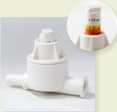
The B-Smart pressure monitor is the first disposable manometer for objective monitoring of injection pressure during administration of peripheral nerve blocks (PNB). Monitoring opening injection pressure with the B-Smart monitor can help identify potentially unsafe injections before they start. When the B-Smart monitor indicates high (> 15 psi) opening injection pressure, the needle can be repositioned and the injection resumed.
