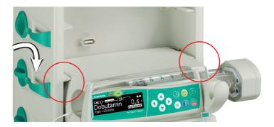
To release, turn the knob clockwise in the vertical position and remove the pump. After release the pump is held in the SpaceStation by the guide rails, but can drop easily due to strong vibrations or during transport.
