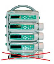
Attention: The operation of a fifth pump mounted under the lowest pump in the system is not allowed.
