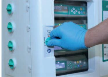
Turn the rotary knob into the door open position and open the door of the SpaceStation MRI.
