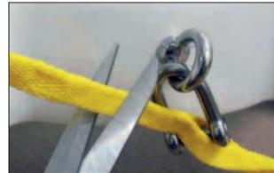
Once the tether is attached and in place cut off the excess line. In order to maintain the integrity and full strength of the tether it is important to leave at least 4 cm / 1.5 inch at the end of the line. Lock the brakes of the four castors/wheels when a safe working distance is indicated by the *Tesla<sup>SPY</sup>*.
