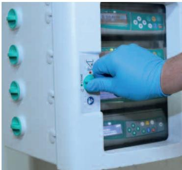
Push the door to close and turn the rotary knob into the horizontal door lock position. Check for acoustic and haptic feedback to ensure that the door is closed.
